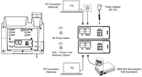
The IP phone should be used with Yealink original power adapter (5V/600mA) only. The use of the third-party power adapter may cause the damage to the phone. If you are connecting a PC to your phone, we recommend that you use the Ethernet cable provided by Yealink.
